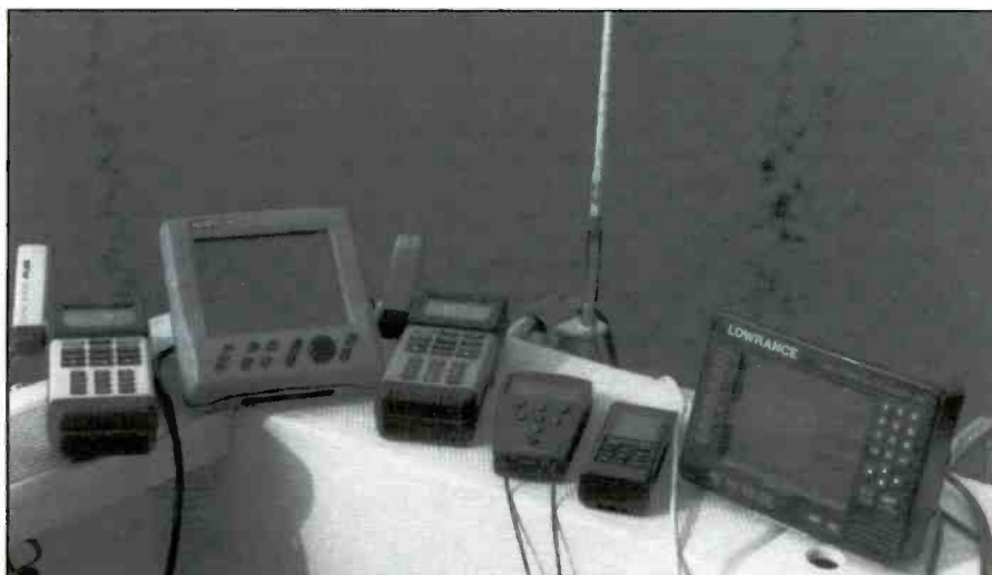
GPS receivers tested with white (center) differential antenna system aboard fish and game patrol boat.
